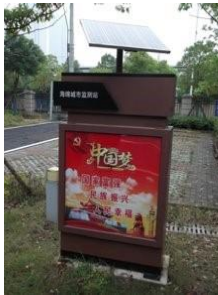
One of the environmental monitoring stations capturing water quantity and water quality data – they are situated at 108 locations across the city
